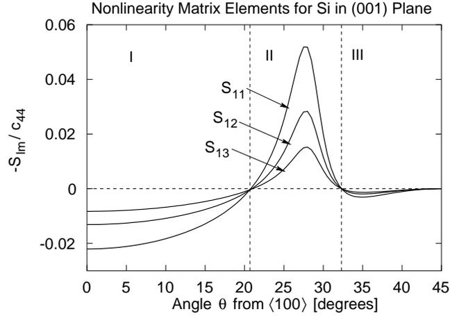
**FIGURE 1.** Nonlinearity matrix elements  $S_{11}$ ,  $S_{12}$ ,  $S_{13}$  for crystalline silicon in the (001) plane as a function of direction. Because of the symmetries of this cut, the matrix elements are symmetric about  $\theta = 45^\circ$  and periodic every  $90^\circ$ . The matrix elements  $S_{lm}$  are normalized by the second-order elastic constant  $c_{44}$ .
